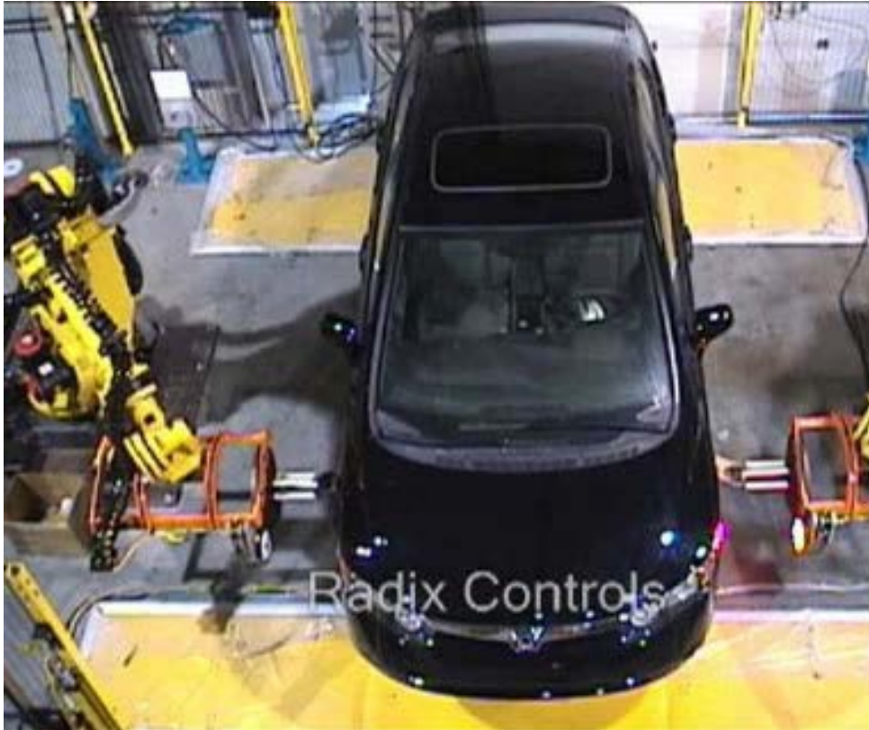
Vision-guided robots position nut runners on wheels
